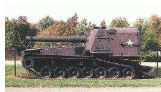
M55 Self-propelled Howitzer Length: 26' Width: 12' Height: 12'
