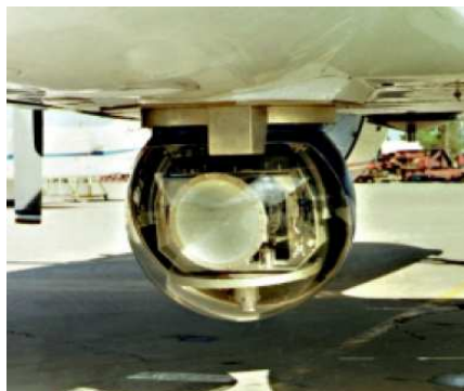
ADTS Radome on belly of Gulfstream G1
