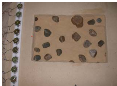
Excavated Scan Region Showing Buried Rock Layout
